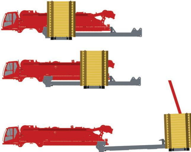
In VPC-MAX configuration, the counterweight tray moves to the end of the VPC-MAX beam prior to beam extension, thus minimizing tailswing and increasing job site mobility.
